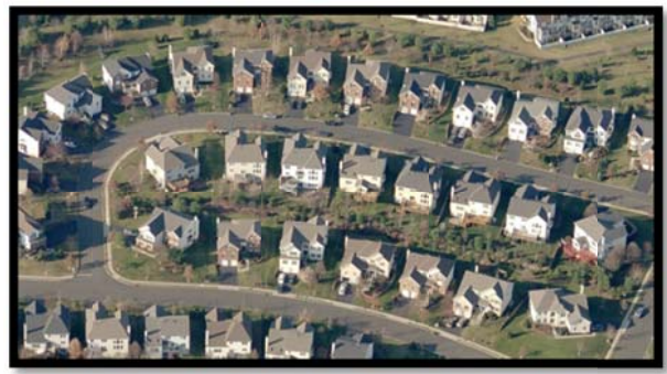
Land Use Code - 1120 Label – “Medium density – single unit” Density - 2-5 units per acre Lot Size - greater than 0.2 acres to 0.5 acres
